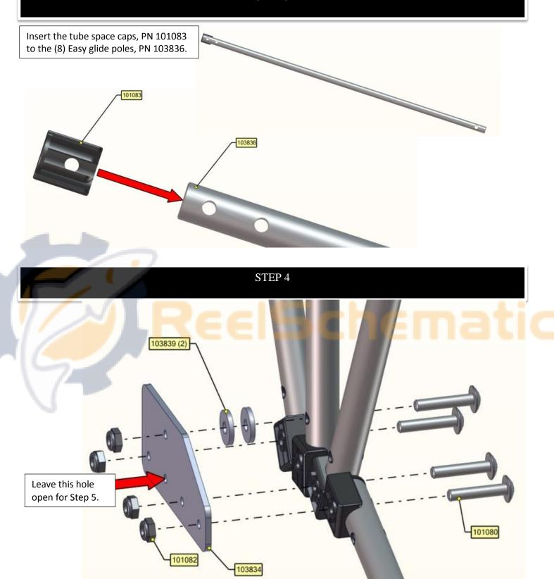
Install the assembled poles from Step 3 to the bracket, PN 103834.
